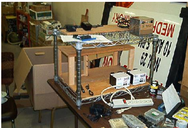
Jay Mudge has fashioned metal shelf housing units to hold DCC power booster and other control units.
